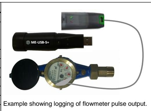
Example showing logging of flowmeter pulse output.
