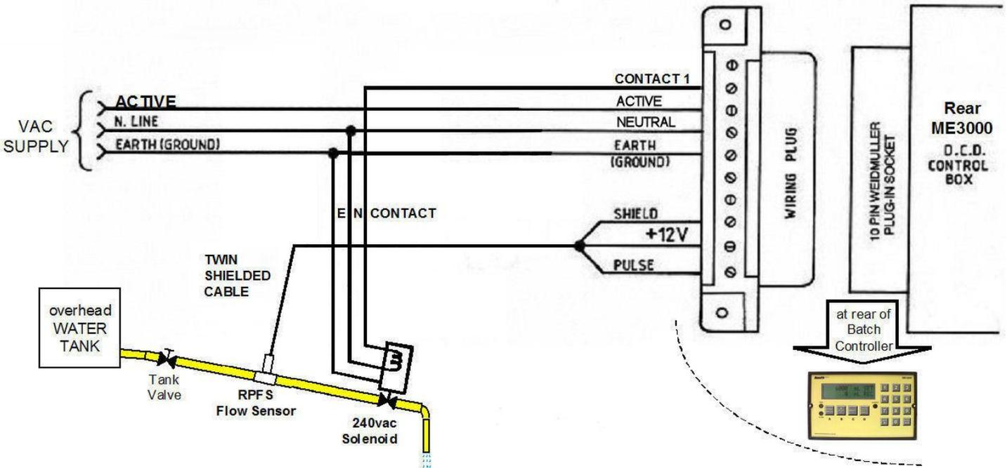
**Wiring for AC Solenoid without Pump**
