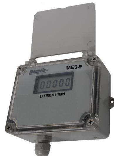
The *ME5-F* digital indicator is designed to operate with most pulse/signal output or coil output flowmeters, providing an instantaneous Flowrate reading in chosen engineering units. Power is via either: an internal Lithium battery which has a typical life of up to 10 years or optional external 5-25 VDC, or 240 vac. The *ME5-F* will accept flowmeter input pulses from 0.2 up to 2000 Hz.
