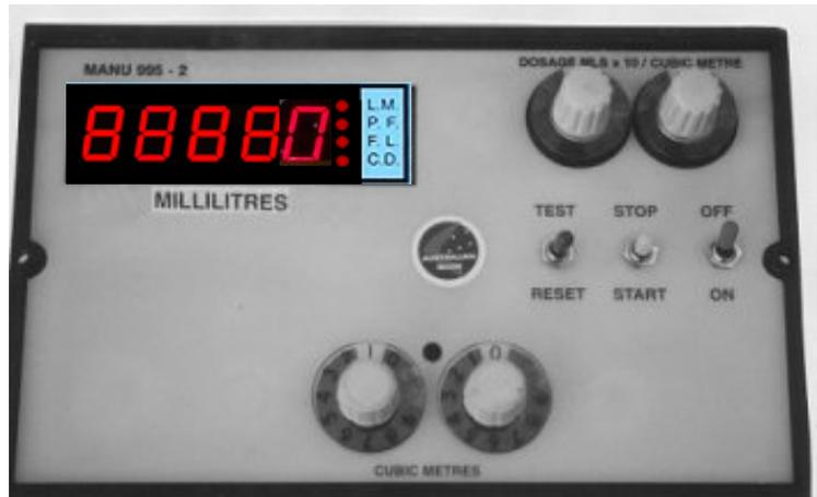
CUBIC METRES preset batch controllers, are designed and used for dosing admixture to comply with quality assurance requirements for the concrete additives industry. It incorporates preact (overflow deduct) feature, allowing speed batching of admixtures with relatively no overruns.
