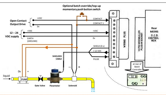
Wiring for DC-powered Batch Controller with DC Open Contact Output Drive to Pump and/or Solenoid
