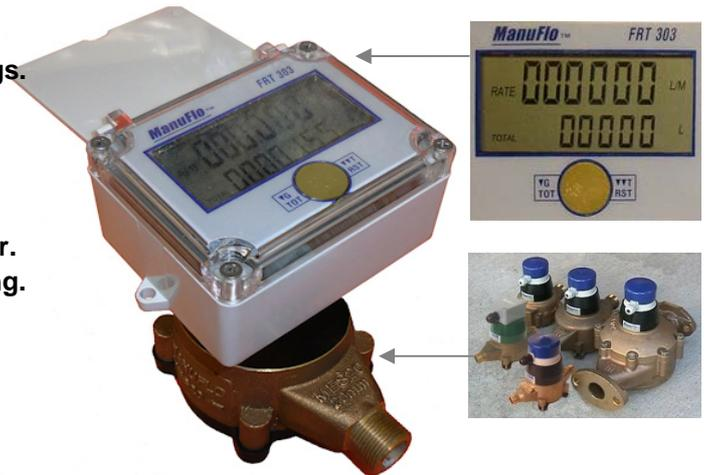
The MES range of nutating disc, magnetically-coupled, positive displacement flowmeters are now available with an integral head readout mounted display version using the FRT303 battery powered indicator.
