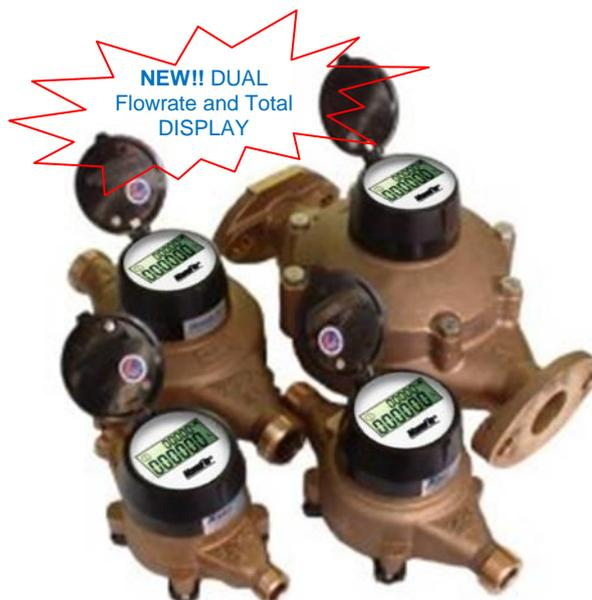
The MESLCD6 series magnetically-coupled positive-displacement flowmeters incorporate an LCD resettable display counter and flowrate meter, powered by an internal long life (5-10 year) Lithium battery. With low to high flowrange performance, the meters are suitable for a wide range of batching and measurement applications for water and water-based chemicals. They are ideal in situations where there is no external power supply available, making them totally portable flowmeters.
