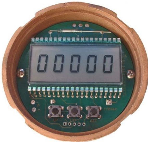
Internal view - PCB and 3 calibration push buttons.
