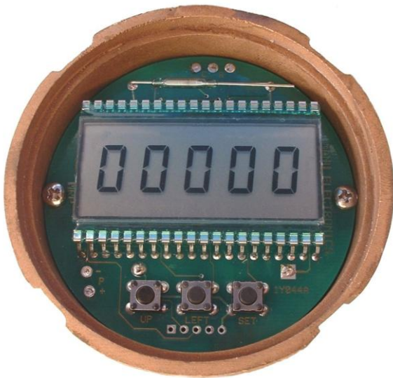
Internal view - PCB and 3 calibration pushbuttons
