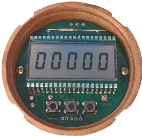
Internal view - PCB and 3 calibration pushbuttons
