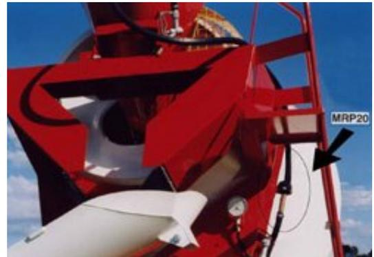
The **MRP20-T2** paddlewheel resettable flowmeter is manufactured by **ManuFlo**<sup>®</sup>, a 100% Australian-owned company with over 45 years experience in flow measurement products. The majority of our products are designed and used for the premix concrete industry. MRP20-T2 resettable flowmeters are tailor-made for the environment of mobile concrete truck mixers (agitators) and plant slumpstands transit mixers / slumpstands.
