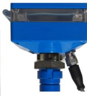
With optional IP67-rated Pulse Output plug set. ≤ 100mm : 1 pulse / Litre; > 110 mm : 1 pulse / 10 Litres
