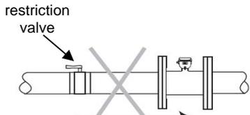
**Possible Problem:** Air pockets, accuracy loss, empty pipe reading
