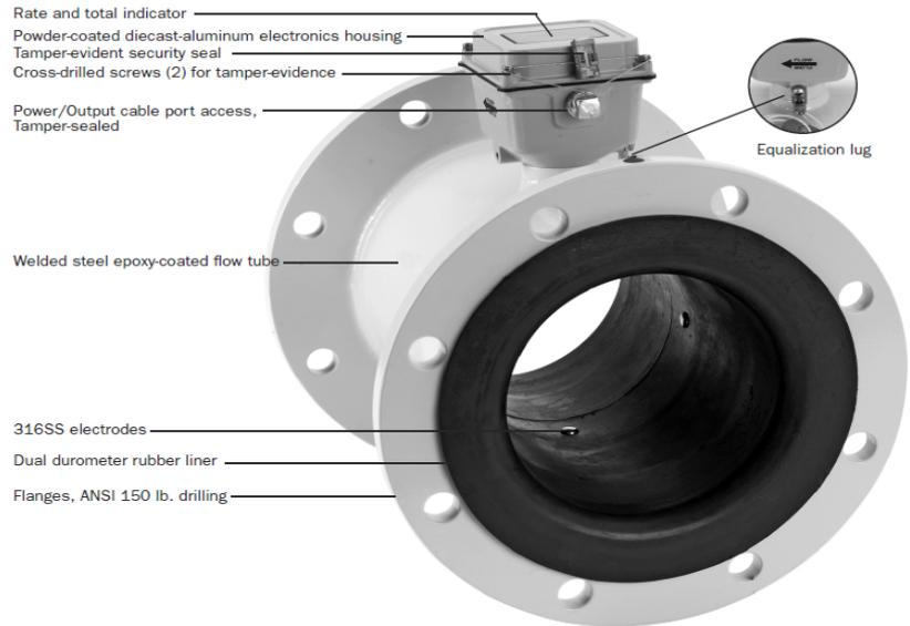
The SM series flowmeters are internal battery powered electromagnetic flowmeters for use in irrigation applications.
