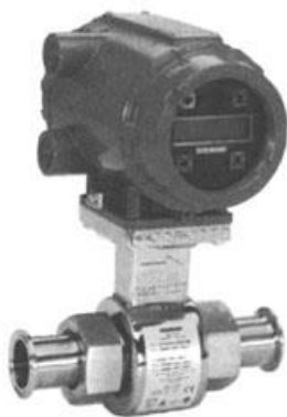
Sanitary Tri-Clamp Stainless Steel sensor lined in PFA (Teflon), with Stainless Steel 316L electrodes, EDPM gasket seals CIP/SIP cleanable, 3-A approved and EL Certified.
