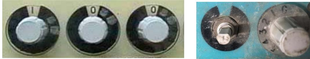
1. The selector knob number dials on the Batch Controller may not be aligned correctly, and therefore do not correspond to the rotary switch numeric values.
