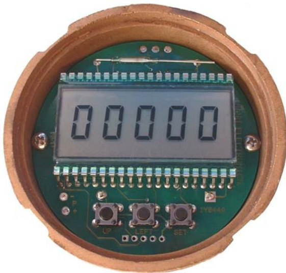
Internal view - PCB and 3 calibration pushbuttons
