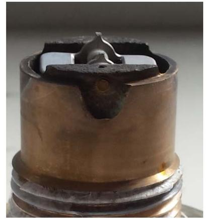
**Paddle wheel has been dislodged from mounting position due to a broken axle**
