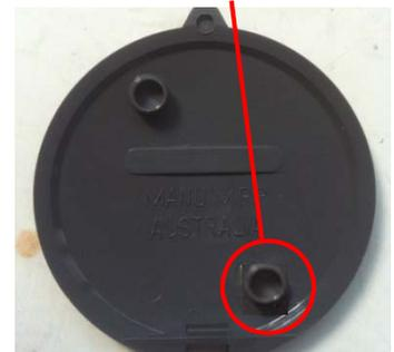
**MRT LCD Locked on 'CAL' message likely caused by moisture ingress**
