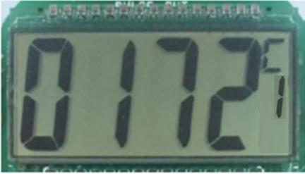
**Flowmeter Display once water flow has stopped 'C1' is indicated
