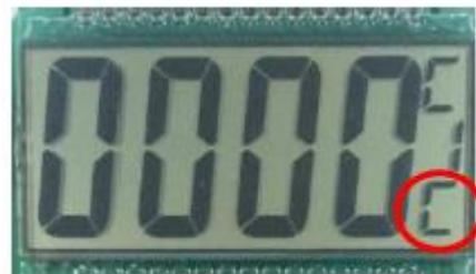
Flowmeter LCD Display in CAL Mode
